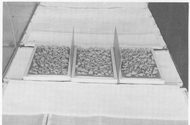
Fig. 1—Photograph of 12.7- to 38-mm clods placed in rain-tower section of wind tunnel before exposure to wind and rainfall.
