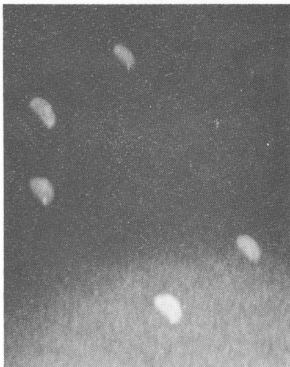
Fig. 1 Here 5 mm drops fall in a 20 mph wind. Wind is blowing from left to right
