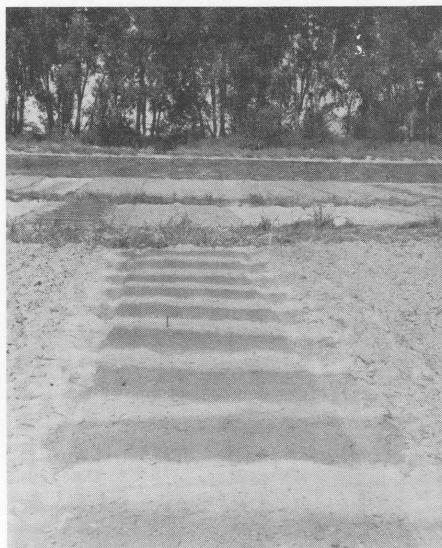
Figure 1. Adhesives applied in, left, 8-inch bands on 40-inch centers; center, 24-inch bands on 40-inch centers; and, right, complete coverage.
