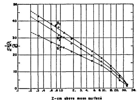
Fig. 1 Local longitudinal-turbulence intensity over rough surfaces
