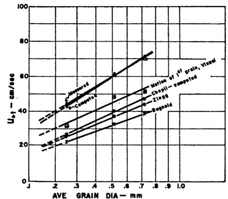
Fig. 5 Threshold friction velocities of several workers compared (abscissa in square-root scale)
