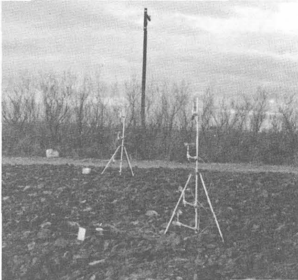
FIGURE 3.—Measuring wind velocities leeward of the tamarisk barrier at the Colby Branch Experiment Station, Colby, Kans.
