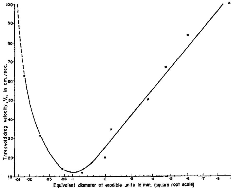
FIG. 2. RELATIONSHIP OF THE THRESHOLD DRAG VELOCITY OF THE WIND TO THE EQUIVALENT DIAMETER OF THE ERODIBLE SOIL UNITS
