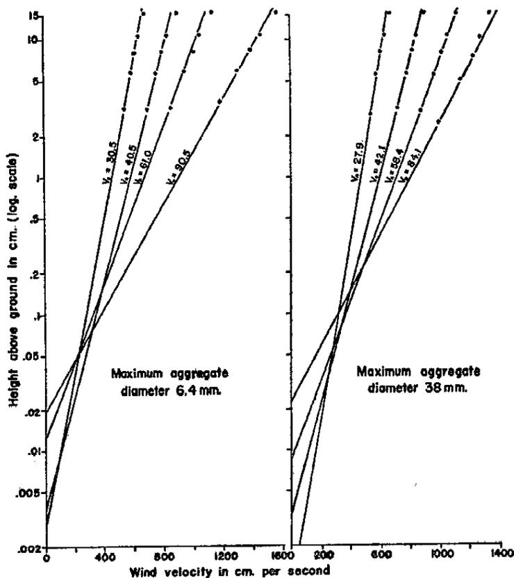
FIG. 1. INFLUENCE OF SIZE OF SOIL AGGREGATES ON WIND VELOCITY DISTRIBUTION AFTER CESSATION OF SOIL REMOVAL
