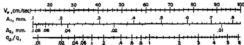
FIG. 3. GUIDE FOR ESTIMATING THE RELATIVE ERODIBILITY ( $q_2/q_1$ ) AND THE MAXIMUM AND MINIMUM EQUIVALENT DIAMETERS ( $A_1$  AND  $A_2$ ) OF ERODIBLE FRACTIONS FROM THE DRAG VELOCITY ( $V_*$ ) OF THE WIND. CORRESPONDING VALUES ARE ALIGNED ALONG A VERTICAL AXIS.
