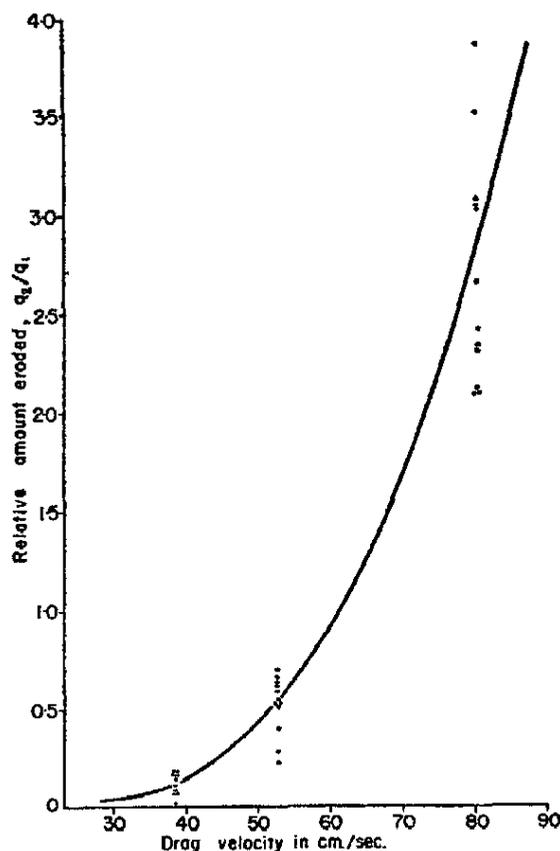
FIG. 4. RELATIONSHIP OF THE RELATIVE AMOUNT OF EROSION TO THE DRAG VELOCITY OF THE WIND
