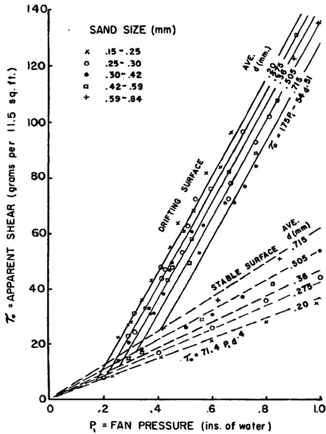
FIG. 6. TRENDS OF APPARENT SHEAR OVER STABLE AND DRIFTING SAND SURFACES IN RELATION TO AN ARBITRARY FAN PRESSURE. THE INTERSECTION OF THE TREND LINES FOR A GIVEN SIZE RANGE OF SAND YIELDS THE SALTATION THRESHOLD SHEAR.
