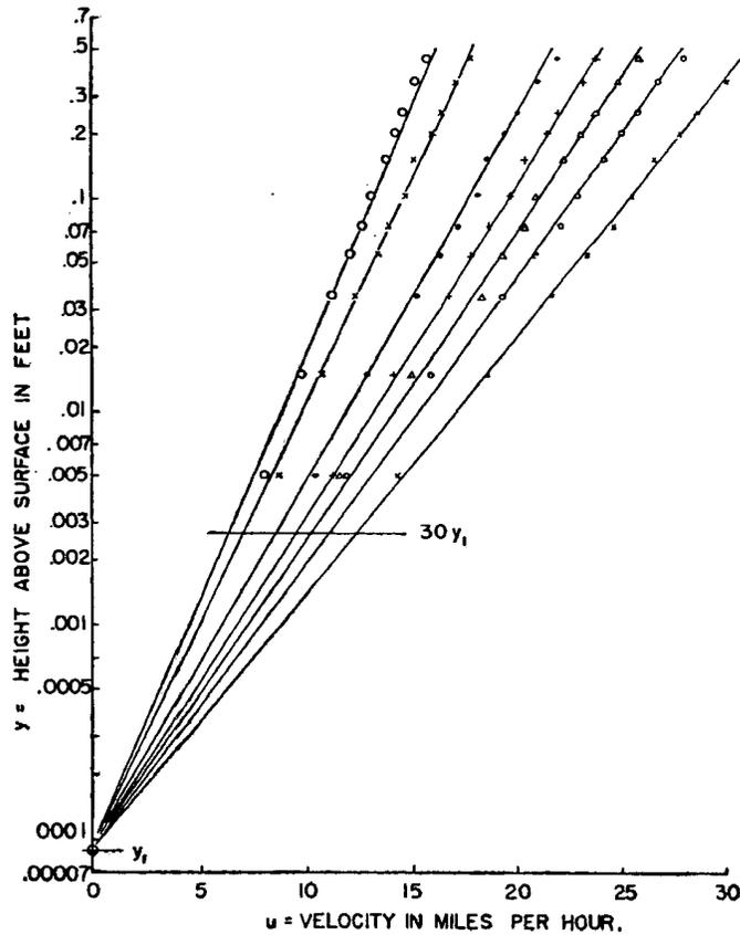
FIG. 1. RELATIONSHIP OF WIND VELOCITY TO HEIGHT ABOVE A 0.30-0.42 MM. STABILIZED SAND SURFACE WITHIN THE TURBULENT BOUNDARY LAYER.
