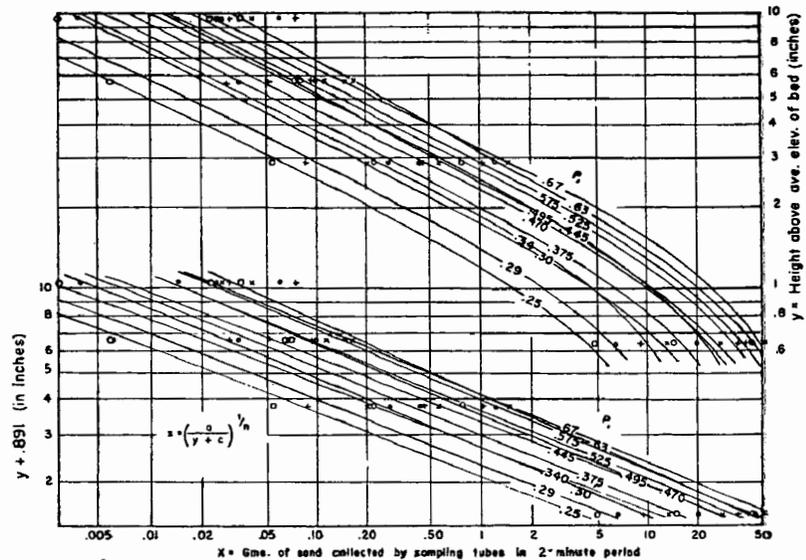
FIG. 8. PLOT OF THE WEIGHT OF SAND COLLECTED BY THE SAMPLER AT FOUR HEIGHTS FOR VARYING PRESSURE LEVELS OF THE FAN.
