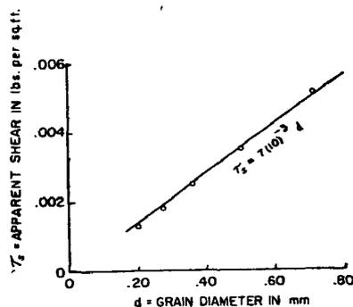
FIG. 7. APPARENT THRESHOLD SHEAR REQUIRED TO INITIATE AND SUSTAIN SAND MOVEMENT FOR A RANGE OF GRAIN DIAMETERS EXCEEDING 0.20 MM.
