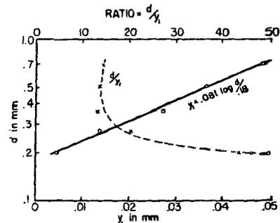
FIG. 3. RELATIONSHIP OF  $y_1$  AND  $d/y_1$  TO AVERAGE GRAIN DIAMETER  $d$ .
