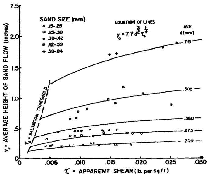
FIG. 9. AVERAGE HEIGHT OF SALTATION SAND MOVEMENT IN RELATION TO APPARENT SHEAR AND SAND SIZE.
