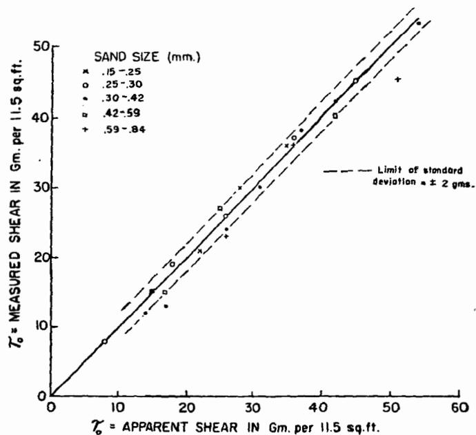
FIG. 2. COMPARISON OF APPARENT AND MEASURED SHEAR VALUES OBTAINED FROM STABILIZED SAND SURFACES OF DIFFERENT RANGES OF SAND.
