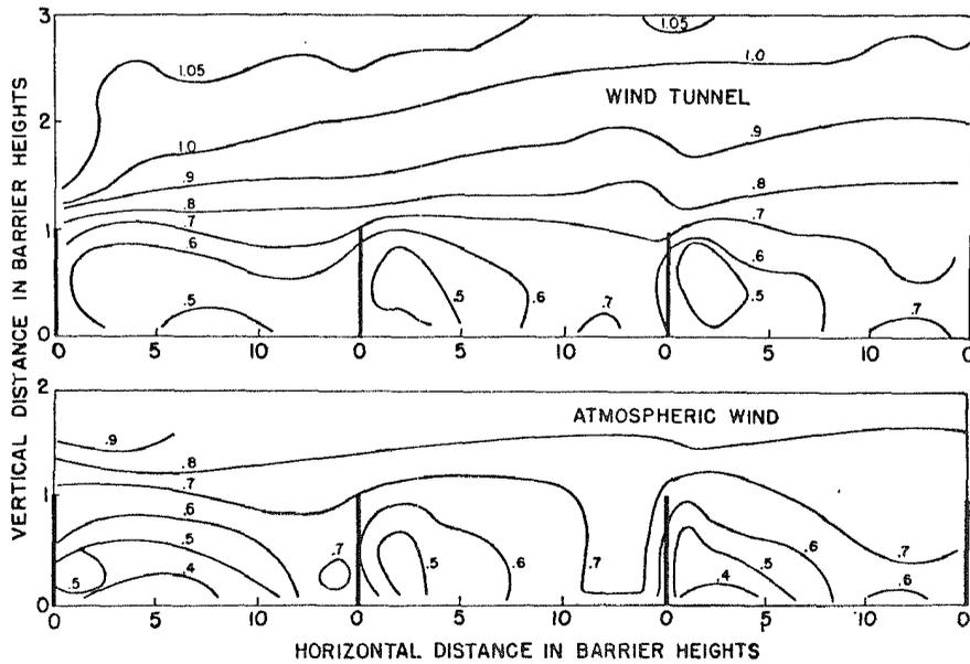
Fig. 3--Velocity ratios  $V_f/V_o$  obtained in vicinity of four successive snow fences placed in the wind tunnel and in atmospheric wind
