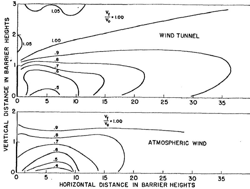
Fig. 2--Velocity ratios  $V_f/V_o$  obtained in vicinity of a single snow fence placed in the wind tunnel and in atmospheric winds
