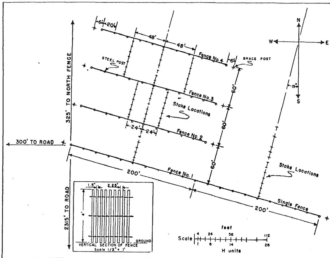
Fig. 1--A map of the snow fence location used to study air-flow patterns
