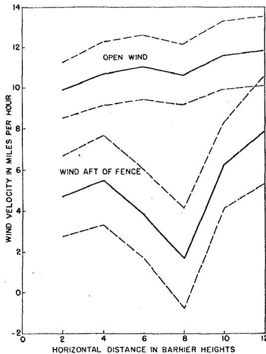
Fig. 6--A comparison of average, maximum, and minimum velocities at the 0.5-ft elevation for open wind and locations aft of a single snow fence; velocities used were obtained from 16h 25m to 17h 25m on May 28, 1953
