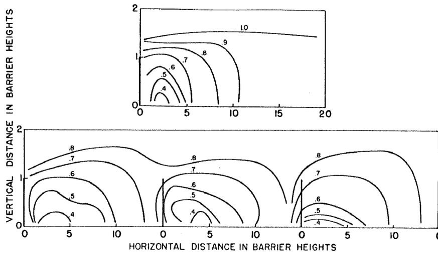
Fig. 4--Velocity ratios  $V_f/V_o$  obtained in vicinity of a single and four successive snow fences placed in oblique atmospheric winds
