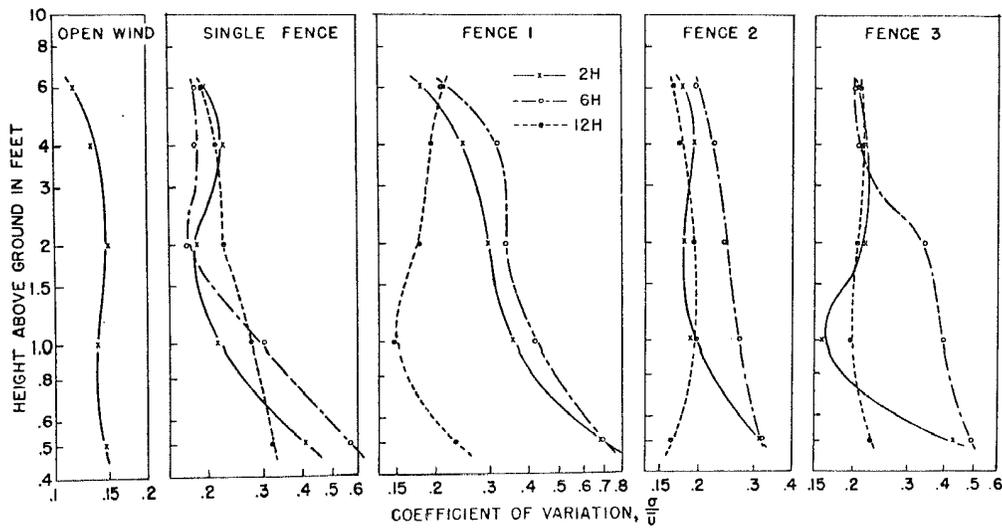
Fig. 5--A plot showing the coefficient of variation  $\sigma/\bar{u}$  at various heights for open winds and for winds aft of single and successive snow fences for one wind from 10h 00m to 17h 25m on May 28, 1953
