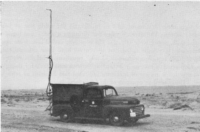
Fig. 1. Atmospheric dust-catching equipment as used in the field. Visibility in this case was 0.55 mile near Menno, Kansas, March 23, 1955.
