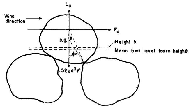
Figure 1—Forces of lift, drag, and gravity acting on a soil grain in a windstream at the threshold of movement of the grain. Net moment opposing  $F_c$  is  $(0.52gd^3\rho' - L_c) \tan \phi'$ .
