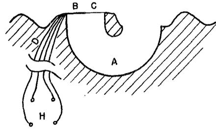
Figure 3—Cross-sectional view of apparatus for measuring lift fluctuations. Direction of wind is normal to the diagram.
