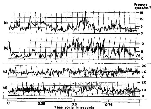
Figure 4—Oscillograph records of pressure of drag and lift on spherical gravel 3.2 and 6.4 mm. in diameter at bed level for a drag velocity of 47 cm. per second: (a) Drag on 3.2 mm. gravel, (b) Drag on 6.4 mm. gravel, (c) Pressure difference between top and bottom of 3.2 mm. gravel, (d) Pressure difference between top and bottom of 6.4 mm. gravel.
