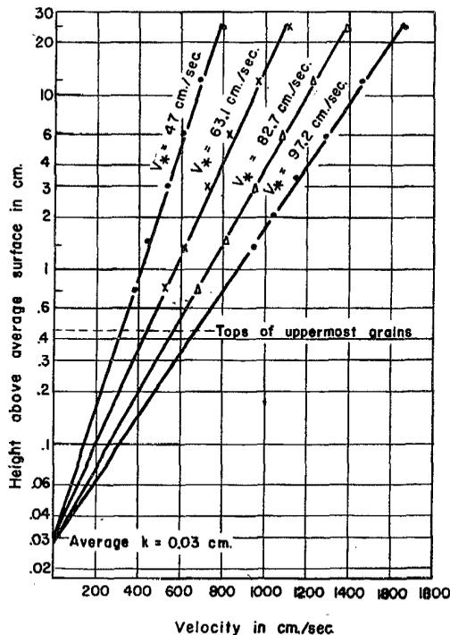
Figure 2—Wind velocity distributions over a smoothed bed of gravel 3.36 to 6.4 mm. in diameter.
