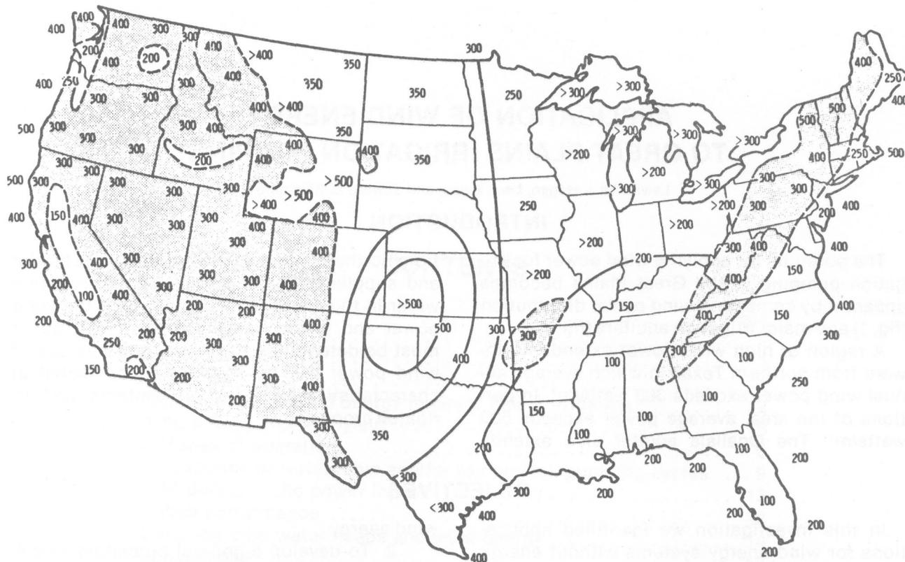
Figure 1.—Mean annual wind power (watts/m<sup>2</sup>) estimated at 50 m above exposed areas. Over mountainous regions (shaded areas), the estimates are lower limits expected for exposed mountain tops and ridges (4).
