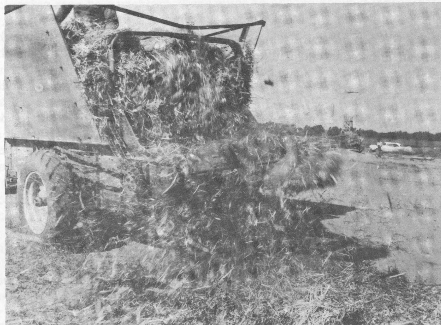
Figure 8.--A beater-type mulch spreader is shown here distributing straw. This type is most suitable for spreading coarse-stemmed stovers such as corn and sorghum. It can be used only on reasonably level ground. (Courtesy of U.S. Corps of Engineers.)
