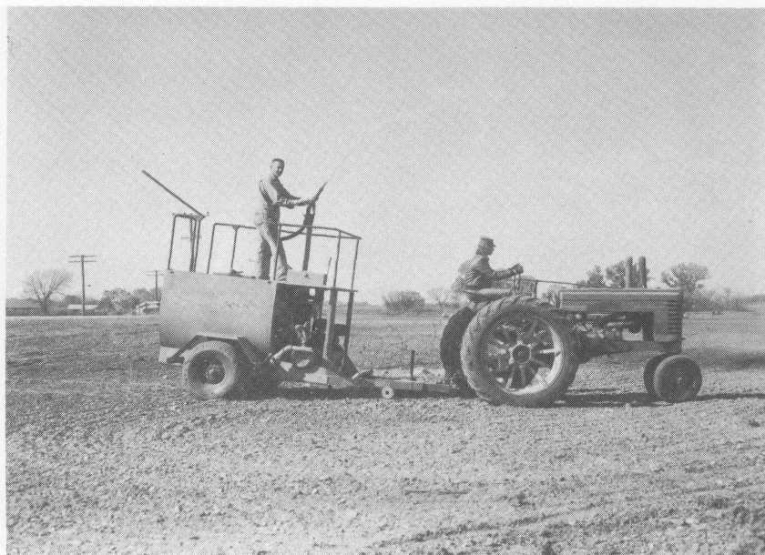
Figure 7.--Hydroseeder sprays seeds and fertilizer mixed with water. The seeder sprays 500 gallons of mixture covering 1 acre in about 15 minutes. Larger units also are available commercially.
