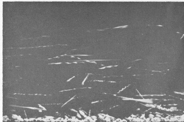
FIG. 2. Photograph of paths of particles moved from left primarily in saltation. The area photographed was 2 by 2 cm (Chepil and Woodruff, 1963, reprinted from Advances in Agronomy , 15, p. 243).
