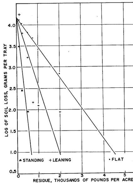
FIG. 2 Effect of wheat-stubble orientation on soil erosion by wind. ( $A = 3.1$  percent clods  $> 0.84$  mm in diameter;  $V = 116.5$  cm per second.)
