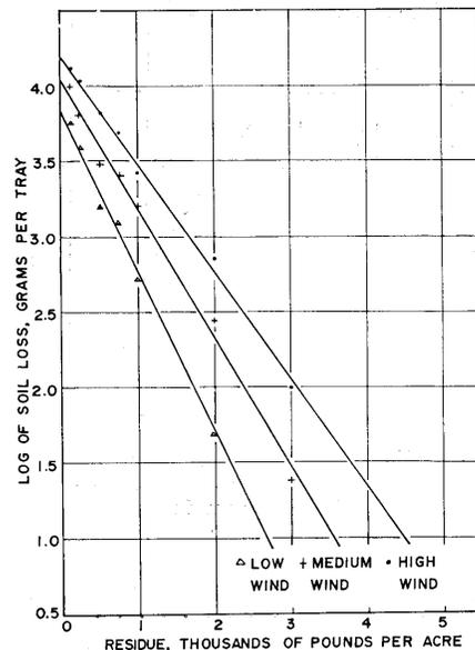
FIG. 1 Effect of wind on soil erosion under a flattened wheat-stubble cover. (A = 3.1 percent clods > 0.84 mm in diameter.)
