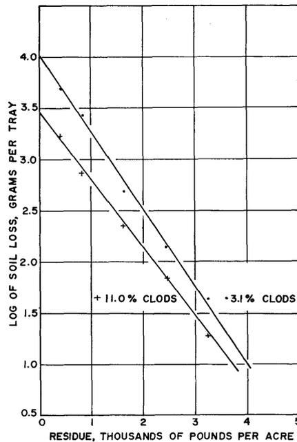
FIG. 4 Effect of soil cloddiness on soil erosion under a leaning, fine-textured sorghum cover ( $V = 105.6$  cm per second).
