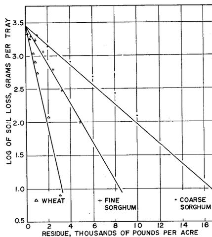
FIG. 3 Effect of kind of residue on soil erosion by wind (orientation = flat, A = 11 percent clods > 0.84 mm in diameter, V = 105.6 cm per second).
