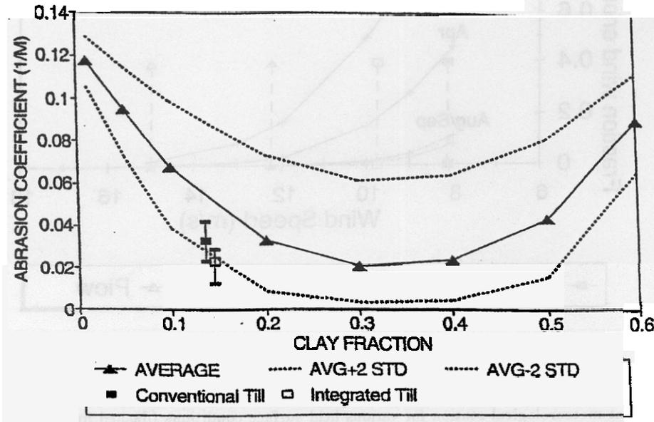
Fig. 6. Calculated mean and standard deviations of clod abrasion coefficients for conventional and integrated tillage on a sandy loam soil in Poland compared to mean and two standard deviations measured in a range of U.S. soils (SKIDMORE and LAYTON 1992, HAGEN et al. 1992)
