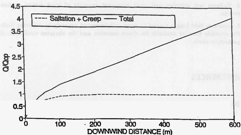
Fig. 7. Simulated saltation and creep downwind horizontal discharge [kg/m] and total downwind horizontal discharge [kg/m] normalized by saltation and creep discharge transport capacity ( $O_{cp}$ ) as a function of downwind field length [m] for a uniform field with conventional-till surface conditions
