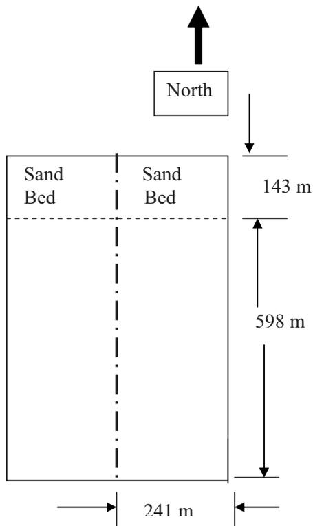
Fig. 2. Schematic of CDF with two sediment storage cells
