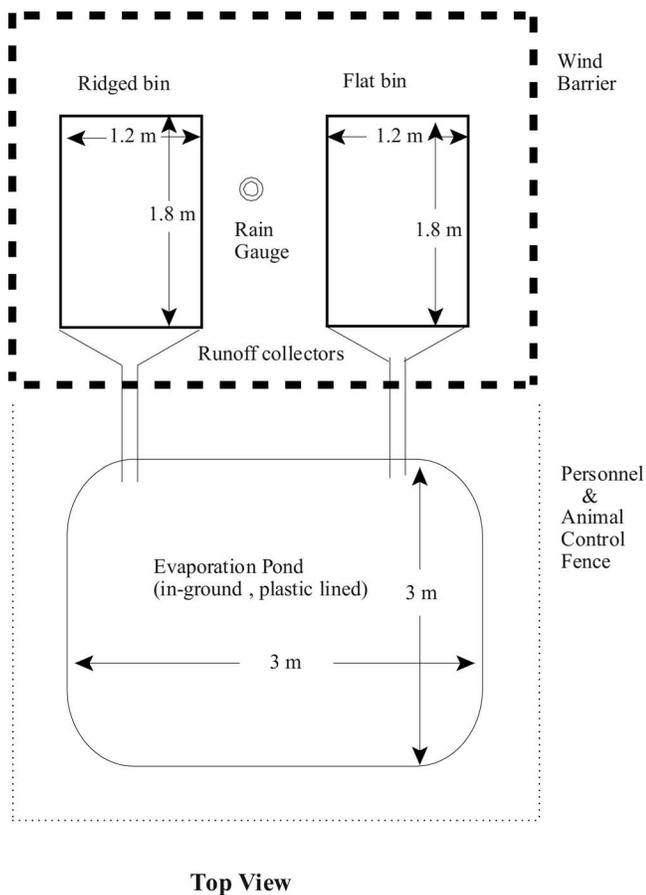
**Fig. 1.** Sediment bins and evaporation pond at Manhattan, Kan. field site
