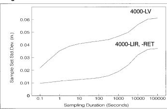
Standard deviation of measurement error (drift) vs. time
