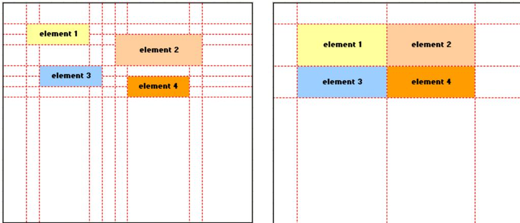
Figure 18-1. Inefficient layout (left) and grid-friendly layout (right)
