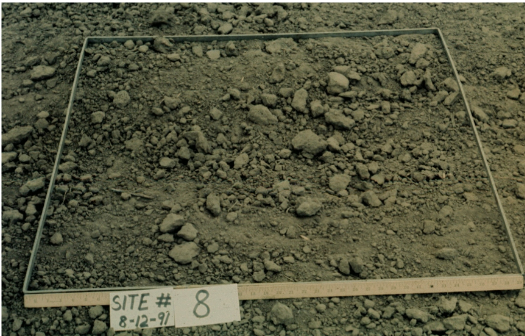
Figure 3.3. Random roughness of 0.40 inches (10 mm).
