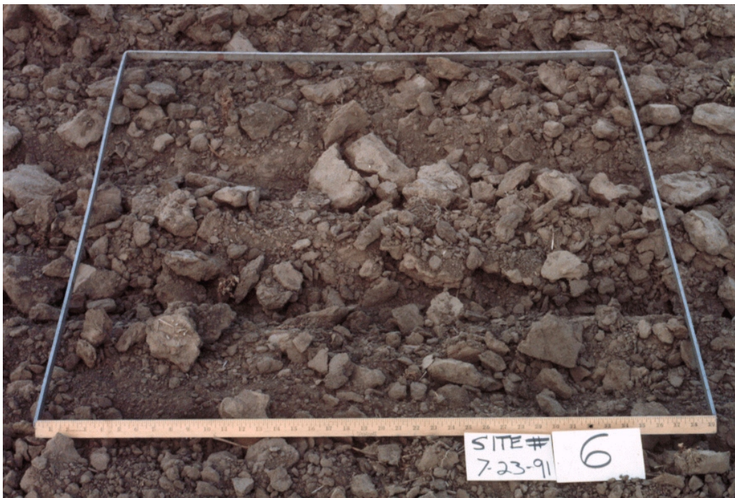
Figure 3.5. Random roughness of 0.75 inches (19 mm).
