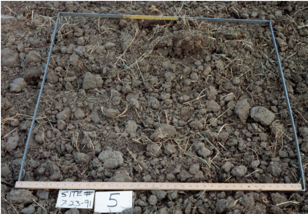
Figure 3.6. Random roughness of 0.85 inches (22 mm).
