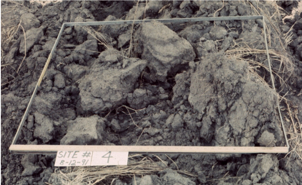
Figure 3.10. Random roughness of 2.15 inches (55 mm).
