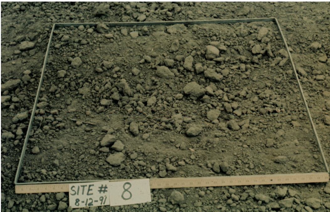
Figure 3.3. Random roughness of 0.40 inches (10 mm).
