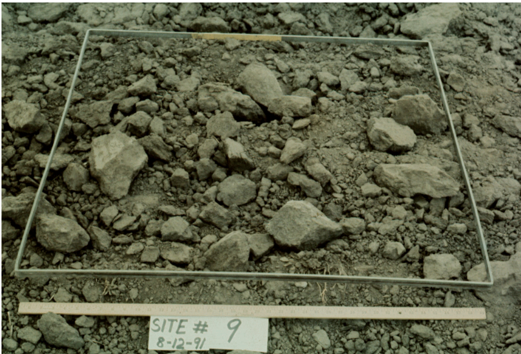
Figure 3.7. Random roughness of 1.05 inches (27 mm).
