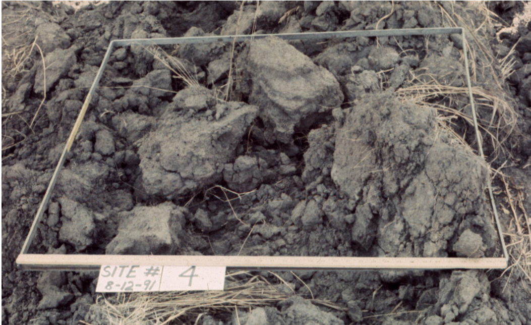
Figure 3.10. Random roughness of 2.15 inches (55 mm).
