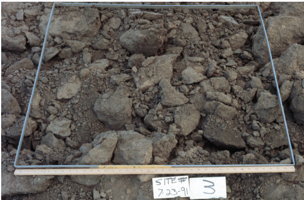
Figure 3.9. Random roughness of 1.70 inches (43 mm).
