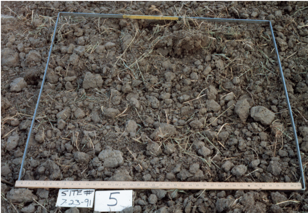
Figure 3.6. Random roughness of 0.85 inches (22 mm).
