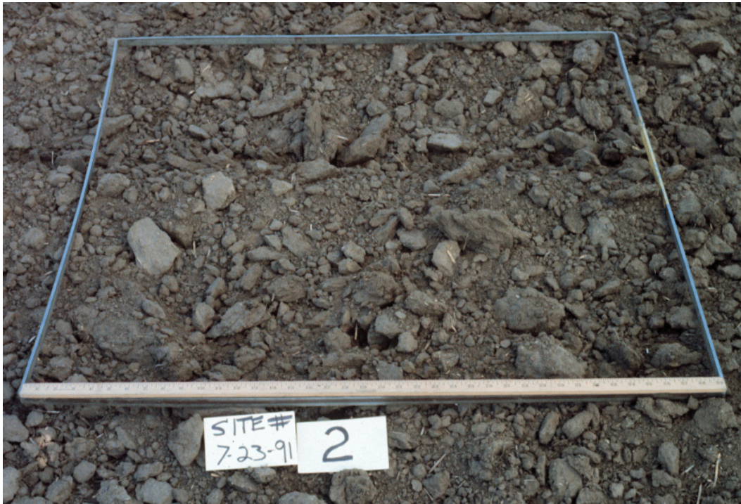
Figure 3.4. Random roughness of 0.65 inches (17 mm).
