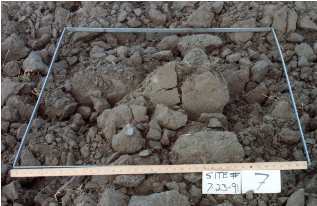
Figure 3.8. Random roughness of 1.60 inches (41 mm).
