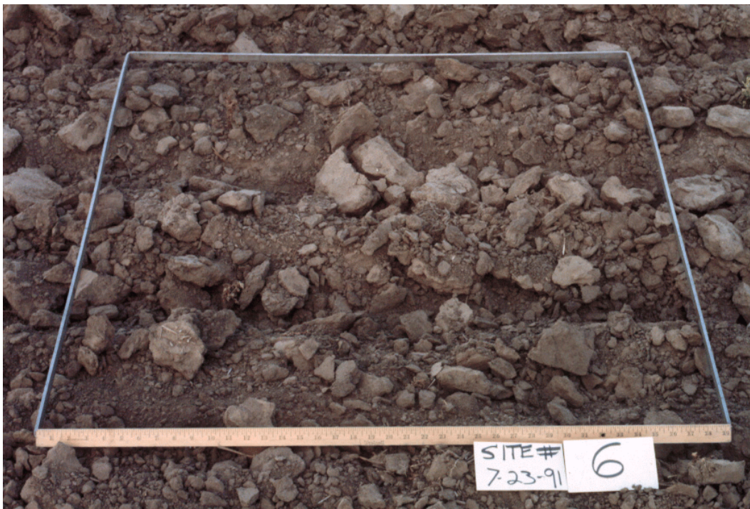
Figure 3.5. Random roughness of 0.75 inches (19 mm).
