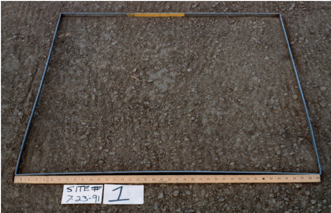
Figure 3.2. Random roughness of 0.25 inches (6 mm).
