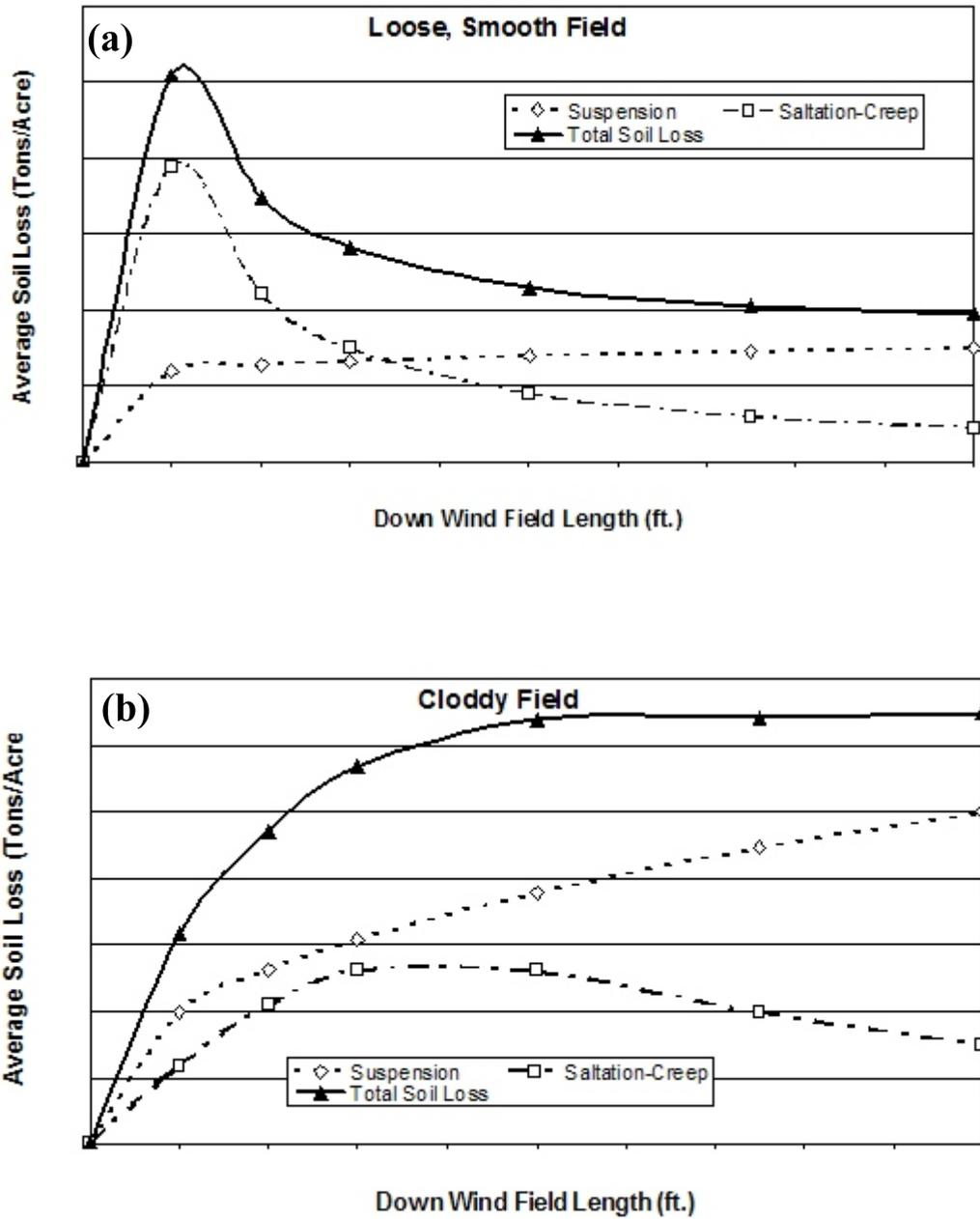
Figure 5.12. Comparison of average soil loss at various downwind distances on (a) a smooth, loose field and (b) a cloddy field.
