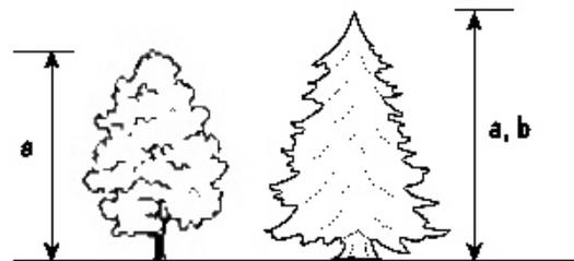
**Figure 5.5.** Barrier height for single-row (a) and multiple-row (b) barriers.
