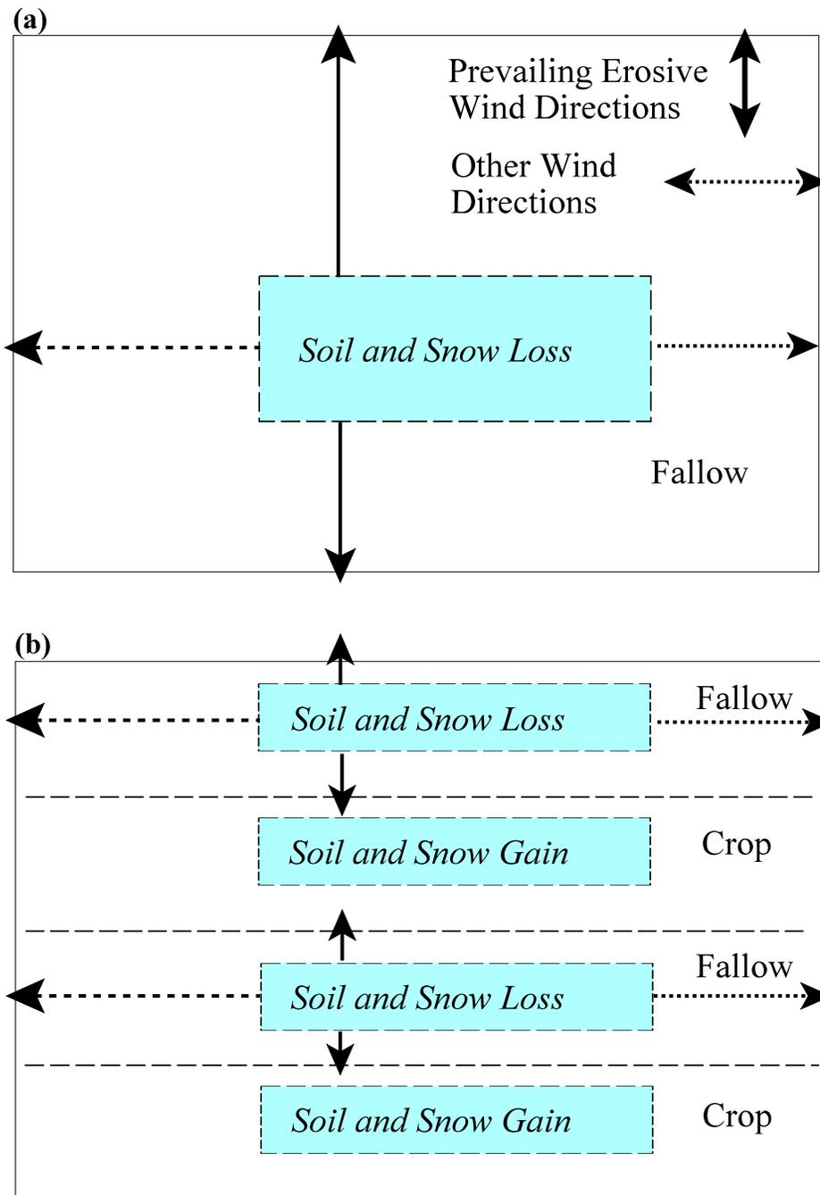
**Figure 5.8.** Comparison of (a) large fallow field and (b) the same field strip cropped with alternating crop and fallow strips.
