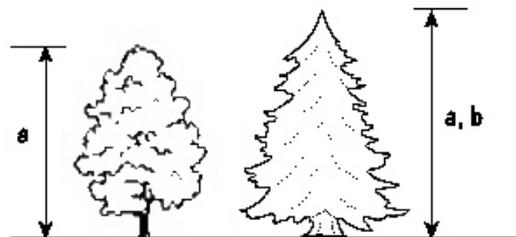
**Figure 3.16.** Barrier height for single (a) and multiple (b) row barriers.
