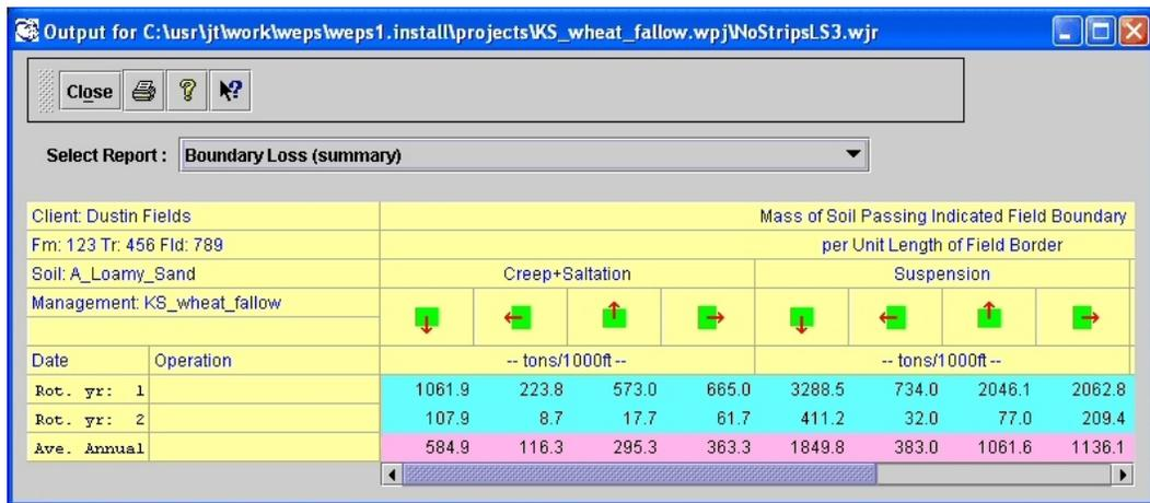
Figure 5.30. Boundary Loss summary for the non-stripped field with a loamy sand soil.
