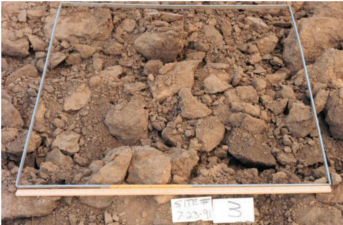
Figure 3-9 Random roughness of 1.70 inches (43 mm).
