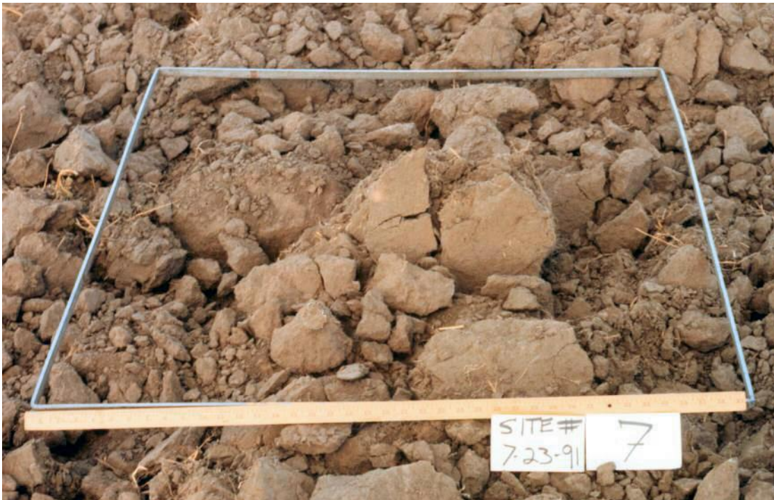
Figure 3-8 Random roughness of 1.60 inches (41 mm).
