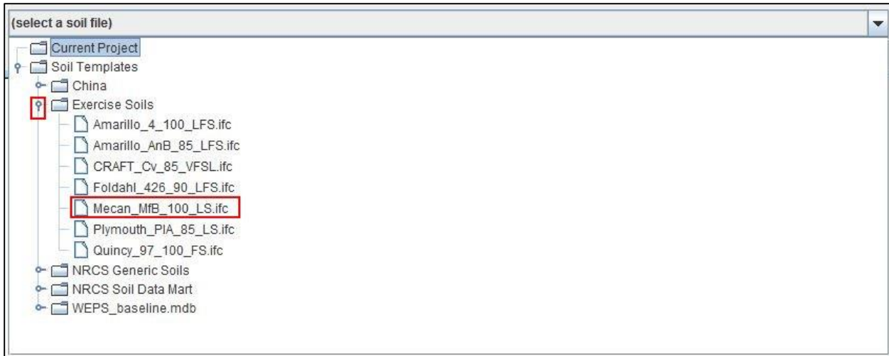
Figure 4-4 Selecting a template (Exercise Soils) soil file using the soil selection drop-down box.
