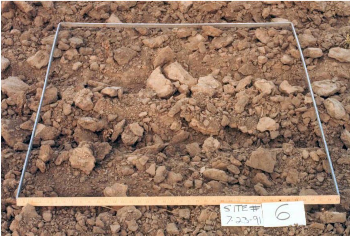
Figure 3-5 Random roughness of 0.75 inches (19 mm).
