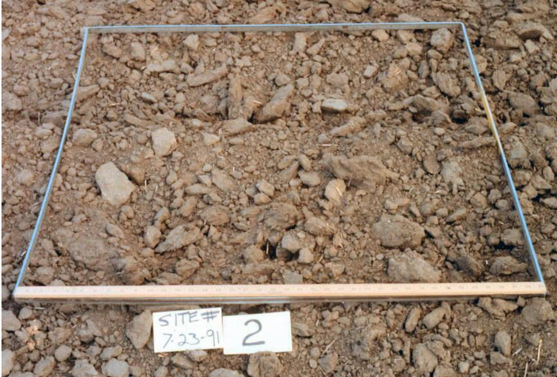
Figure 3-3 Random roughness of 0.40 inches (10 mm).
