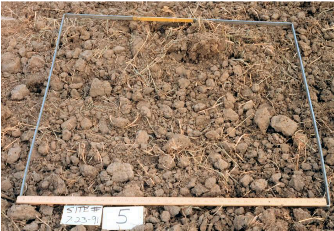
Figure 3-6 Random roughness of 0.85 inches (22 mm).
