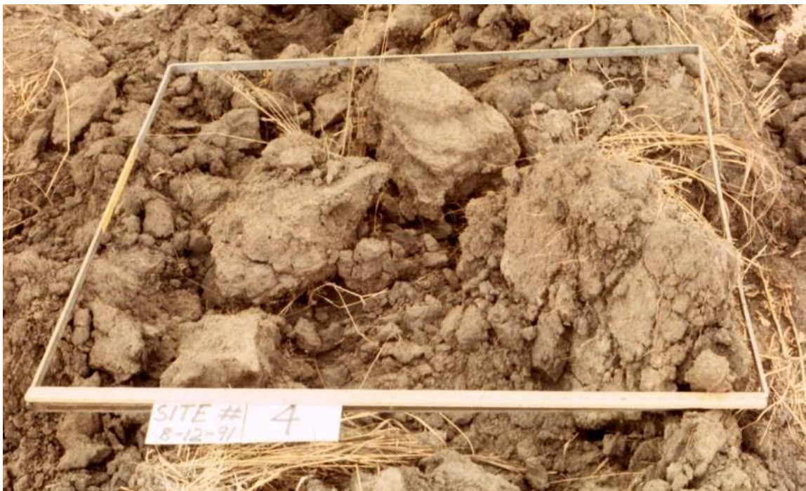
Figure 3-10 Random roughness of 2.15 inches (55 mm).
