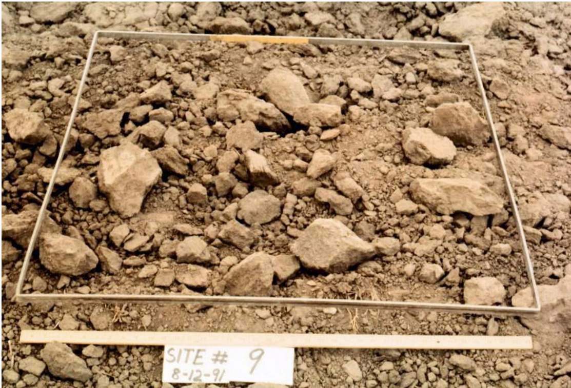
Figure 3-7 Random roughness of 1.05 inches (27 mm).
