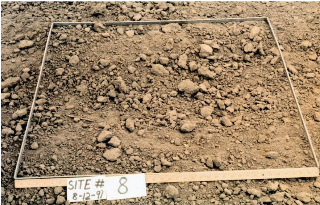
Figure 3-4 Random roughness of 0.65 inches (17 mm).
