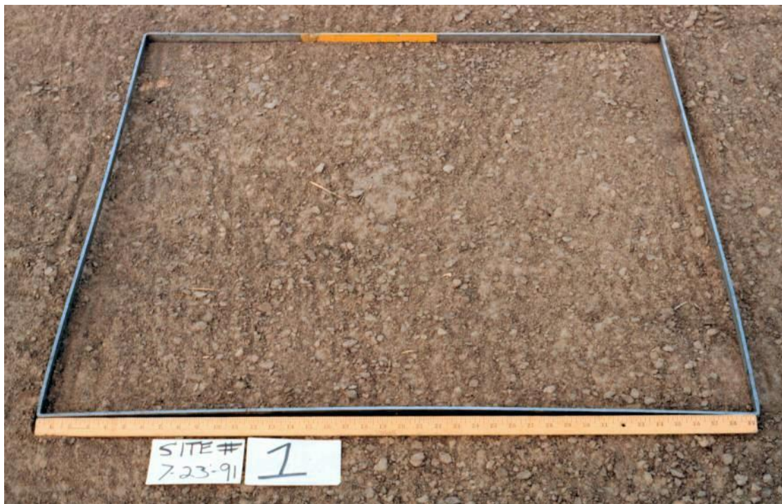
Figure 3-2 Random roughness of 0.25 inches (6mm).
